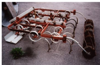
Plate 2. Finnish Tume harrow with rotating tool bars.
