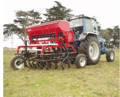
Flexi intermediate plot / farmer carrier frame with spring mounted tool bar assembly Flexi farmer drill fitted with Thian seed box ( www.thianagri.co.nz )
