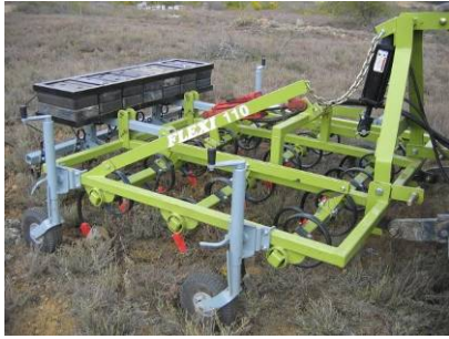
Flexi light frame – test bed trailing and 3 point linkage
