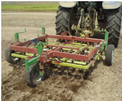
Flexi intermediate plot / farmer carrier frame with spring mounted tool bar assembly Flexi farmer drill fitted with Thian seed box ( www.thianagri.co.nz )
