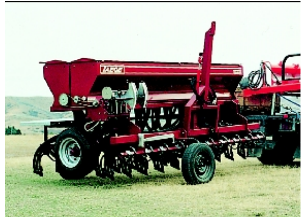
Fig. 8. Double box drill (Model 360 MD) fitted with end-tow (farmer version).
