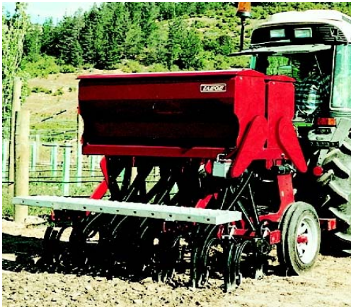
Fig. 5. Vineyard / Plot drill (Model 1.4 ED) direct seeding. “Knife-like” boot shown as insert (B. Taege).
