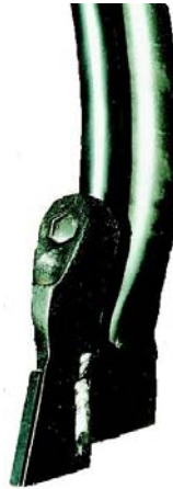
Fig. 5. Vineyard / Plot drill (Model 1.4 ED) direct seeding. “Knife-like” boot shown as insert (B. Taege).
