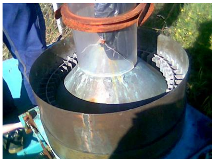
Plate 1. Oyjord cell wheel fitted with extended lamellae fabricated from sheet metal using modified design of Hallerström, 1974..
