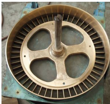
S&N Deep walled (23mm) cell wheel and cone retro-fitted to original Oyjord-Shou planter base plate Plate 3. Cell wheel module which is either manual drive or digital (see Fraser et.al. 2008).
