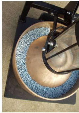
320 cell wheel loaded with 1kg fert. Note uhmwpe-BR base plate
