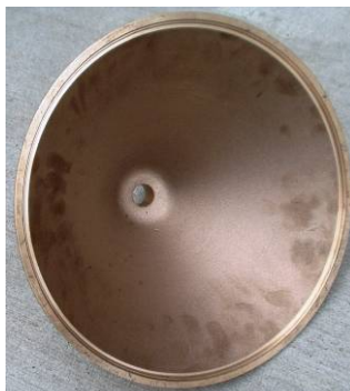
S&N Deep walled (23mm) cell wheel and cone retro-fitted to original Oyjord-Shou planter base plate Plate 3. Cell wheel module which is either manual drive or digital (see Fraser et.al. 2008).
