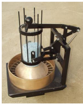
320 mm cone – 1kg fert. Tube 110 mm ID x 250mm
