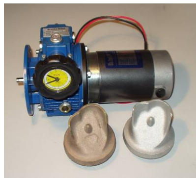
Plate 3. Direct coupled dynamo fitted with inverse impellor (left) and standard distributor impellor blocks (right) cast in bronze and aluminium with raised centre. High performance Brooks – S & N 12v drive plus in-line mechanical variator in background.
