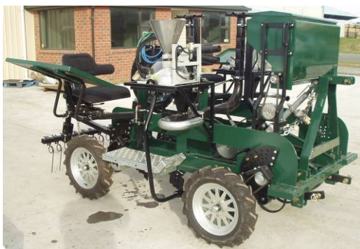
Plate 2. S&N Flexi Plot Seeder fitted with Kincaid cones.
