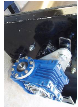
Brooks right-angle drive 7.5:1 and 15:1 ratio plus torque arm
