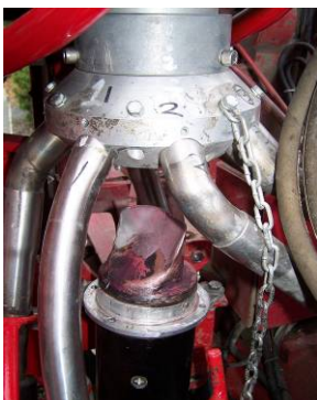
Plate 3. Direct coupled dynamo fitted with inverse impellor (left) and standard distributor impellor blocks (right) cast in bronze and aluminium with raised centre. High performance Brooks – S & N 12v drive plus in-line mechanical variator in background.
